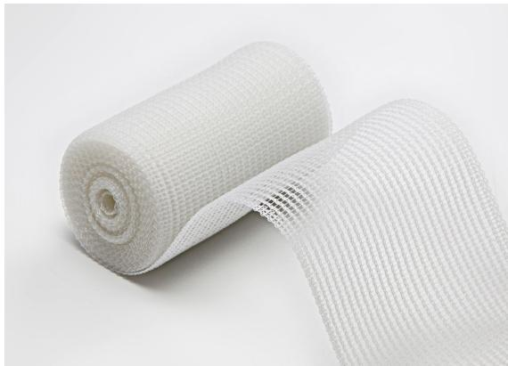
Gauze-flex is used to create insulation distance around the conducting parts when making an injection joint. It also contributes to an optimal distribution of the resin in the injection joint. Because of the width, the 10 cm wide version is very suitable for the insulation of the earth screen as well as for wrapping up the total joint.
