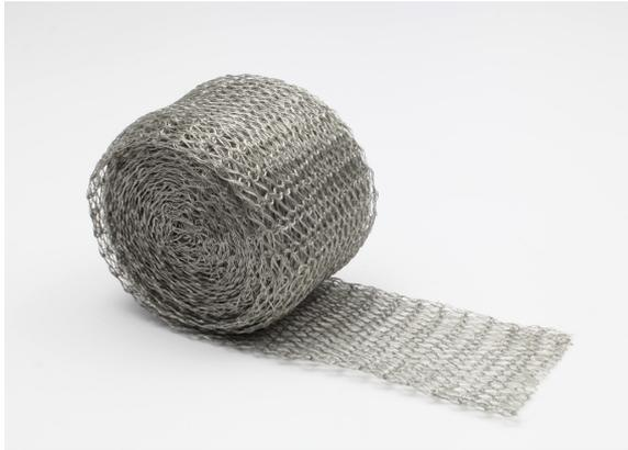
Copper wire mesh is used for shielding and earthing in telecommunication joints and others. The wire mesh needs to be applied with a slight tensile force, without pleats, and with half overlap. Both ends of the wire mesh need to be fixed with a constant force spring or by soldering.
